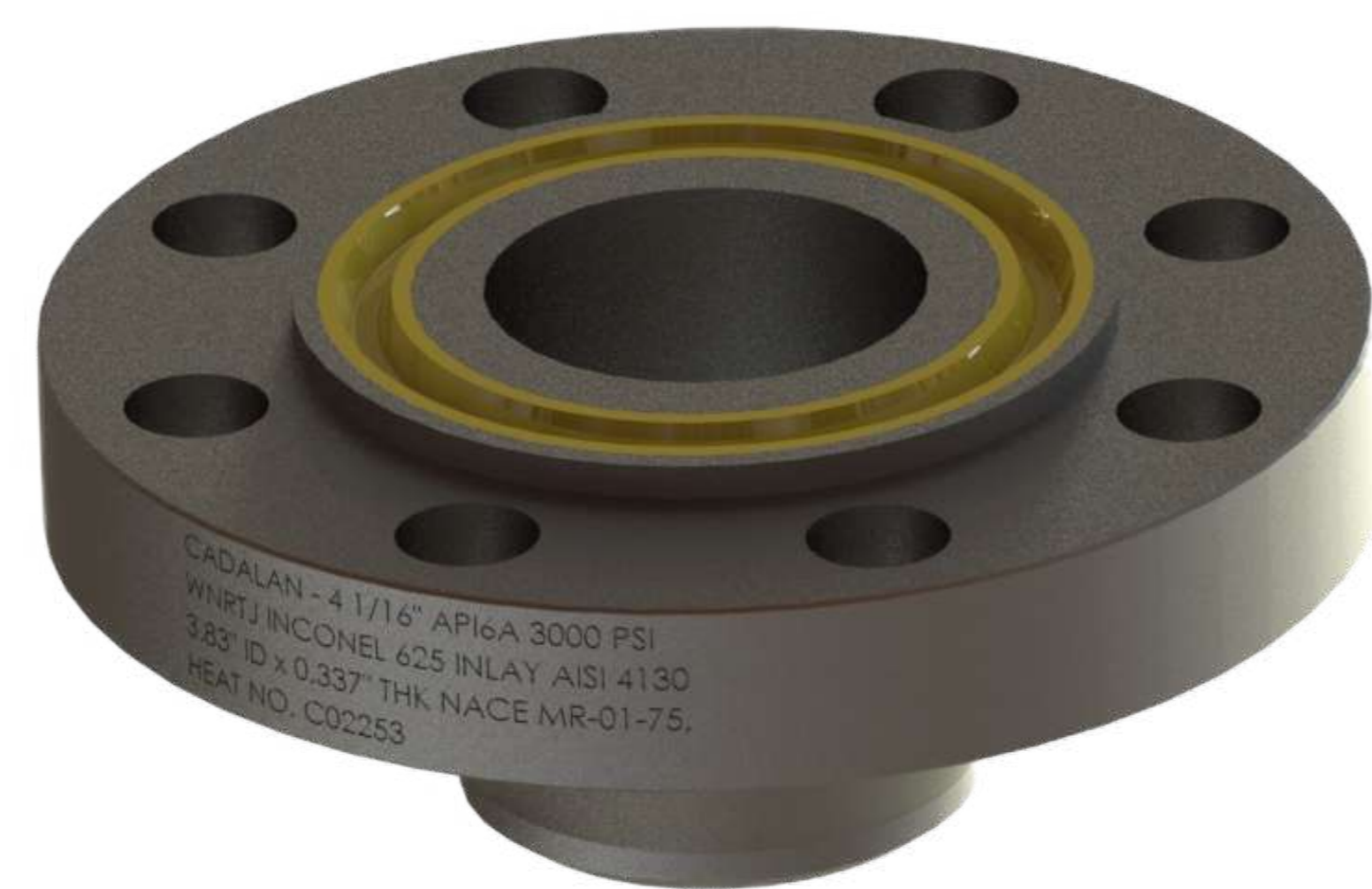
WELD OVERLAY FLANGES (INCONEL 625 INLAY) BASE MATERIAL : CARBON STEEL, HYCS, ALLOY STEEL INLAY / OVERLAY : SS316/ INCONEL 625
